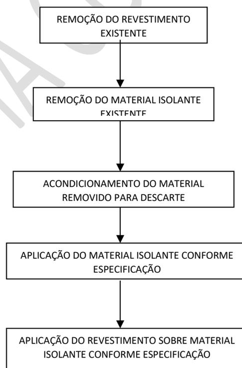
**2.1.1.5 FLUXOGRAMA DO PROCESSO PRODUTIVO DA RISOTERM – REVESTIMENTO REFRAATÁRIO**
